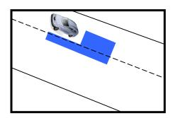
2. Avoid patches within existing patches. If this cannot be avoided, make the boundaries of the patches coincide.
