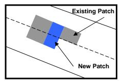
**3.** Asphalt and concrete pavements should be removed by saw cutting or grinding. Avoid breaking the edges of the existing pavement or damaging the remaining pavement with heavy construction equipment.
